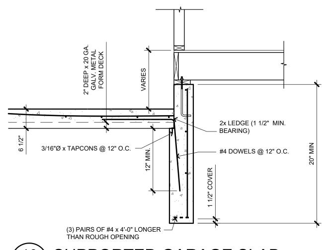
SUPPORTED GARAGE SLAB SCALE: 3/4" = 1'-0"
