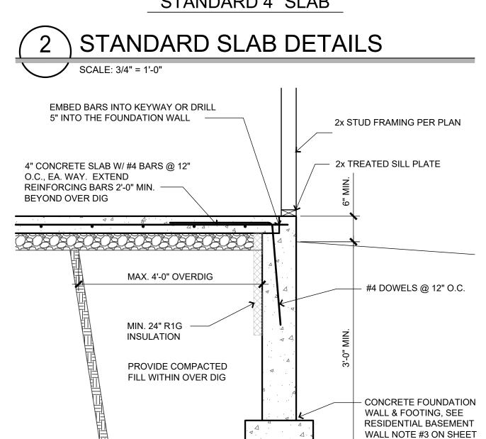
OVERDIG SECTION BSMT SLAB SCALE: 3/4" = 1'-0"
