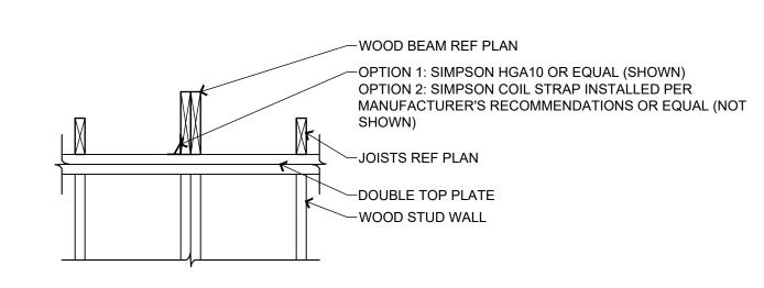
TYP WOOD BM PERP TO WALL SCALE: 3/4" = 1'-0"
