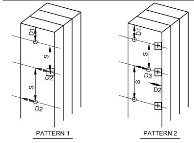
CONTRACTOR MAY SUBSTITUTE 1/2"Ø BOLTS W/ METAL PLATE OR WASHER IN PLACE OF 30d & 50d CONTRACTOR SHALL PRE-DRILL STUDS W/ 1/8" DRILL BIT WHEN USING 30d & 50d NAILS TO PREVENT SPLITTING. ALL BUILT UP COLUMNS SHALL EXTEND TO THE ROOF TRUSSES
