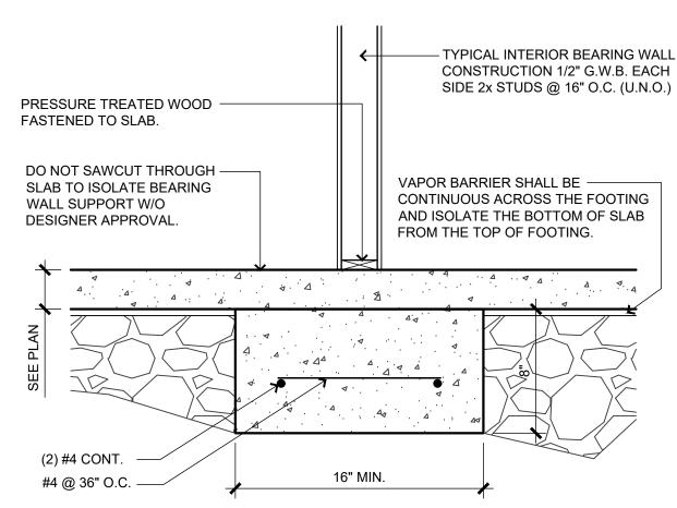
INTERIOR BEARING WALL SCALE: 3/4" = 1'-0"
