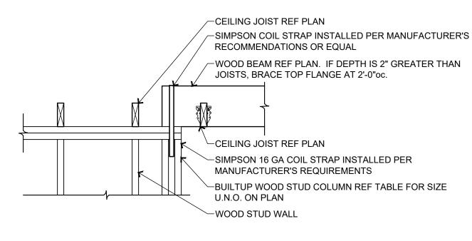
TYP WD BM PARALLEL TO WALL SCALE: 3/4" = 1'-0"
