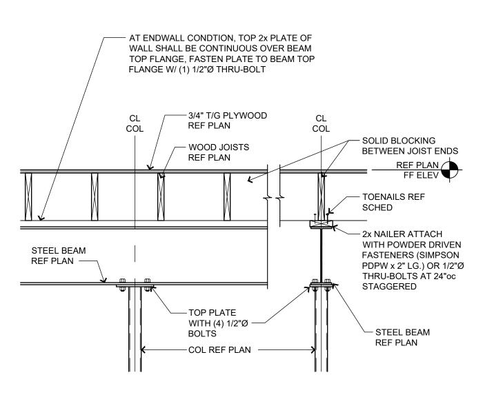
TYP. BEAM AT COLUMN SCALE: 3/4" = 1'-0"
