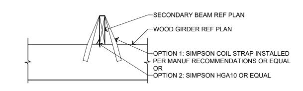
WD BM BEARING ON WD BM SCALE: 3/4" = 1'-0"
