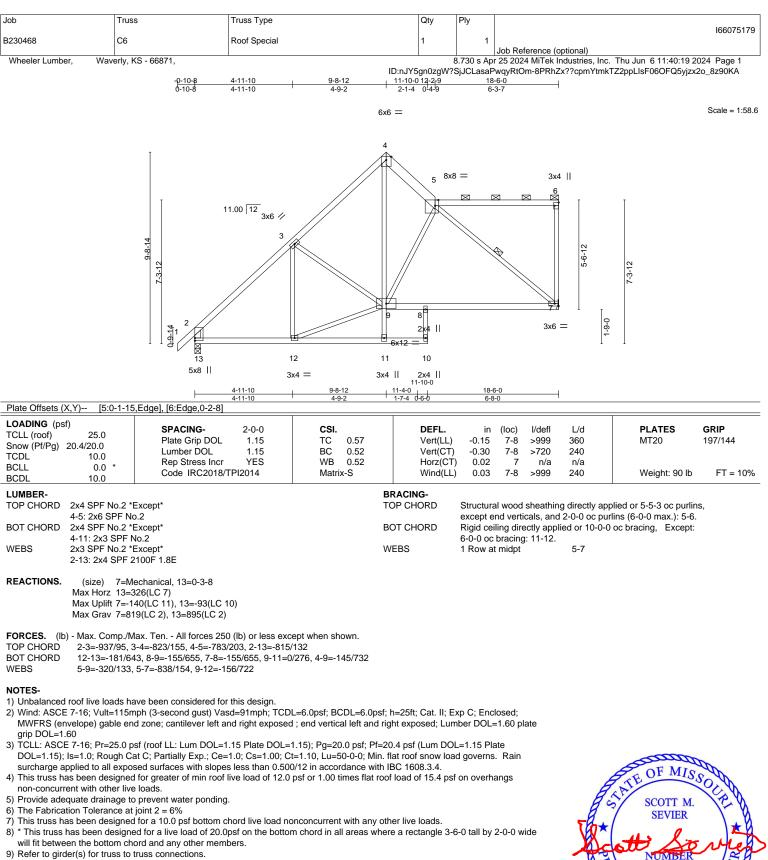
Refer to girder(s) for truss to truss connections.
