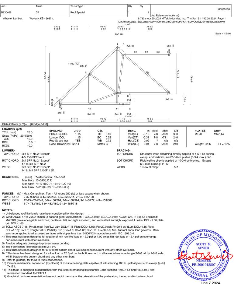
11) This truss is designed in accordance with the 2018 International Residential Code sections R502.11.1 and R802.10.2 and referenced standard ANSI/TPI 1.
