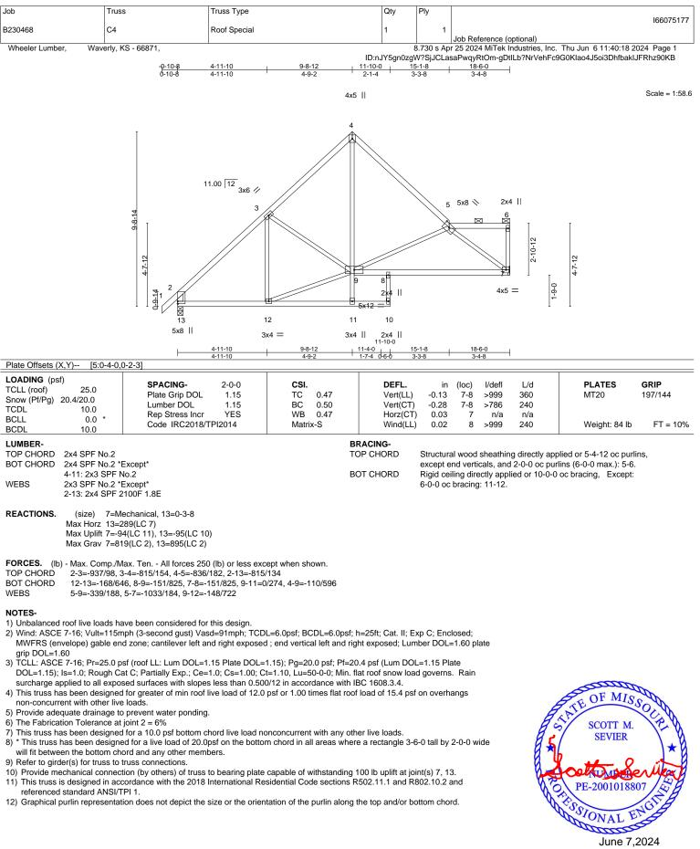
WARNING - Verify design parameters and READ NOTES ON THIS AND INCLUDED MITEK REFERENCE PAGE MII-7473 rev. 1/2/2023 BEFORE USE. Design valid for use only with MiTek® connectors. This design is based only upon parameters shown, and is for an individual building component, not and BCSI Building Component Safety Information available from the Structural Building Component Association (www.sbcscomponent.com)
