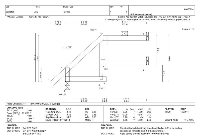
WEBS 2x3 SPF No.2 **REACTIONS.** (size) 4=Mechanical, 9=0-3-8, 5=Mechanical Max Horz 9=102(LC 10)
