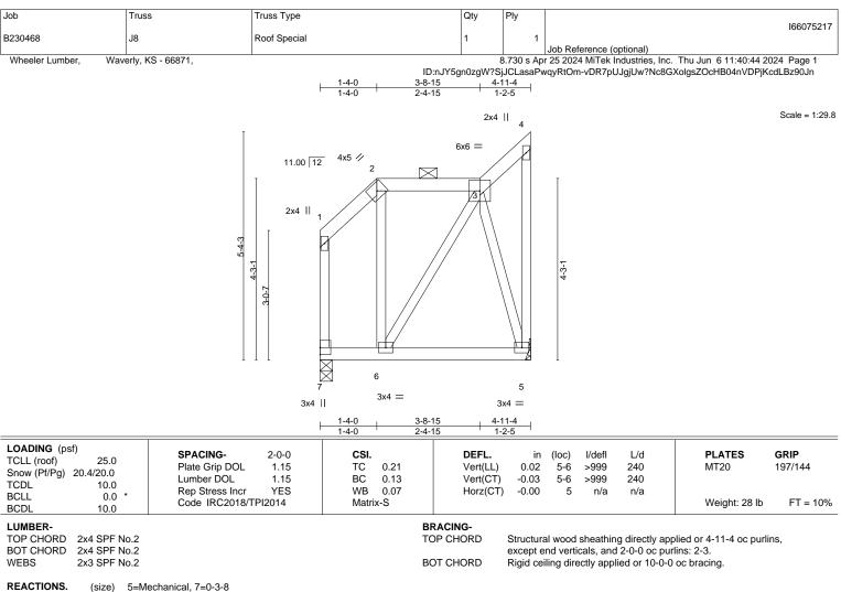
Max Horz 7=191(LC 7) Max Uplift 5=-98(LC 7), 7=-61(LC 6) Max Grav 5=224(LC 21), 7=238(LC 22)
