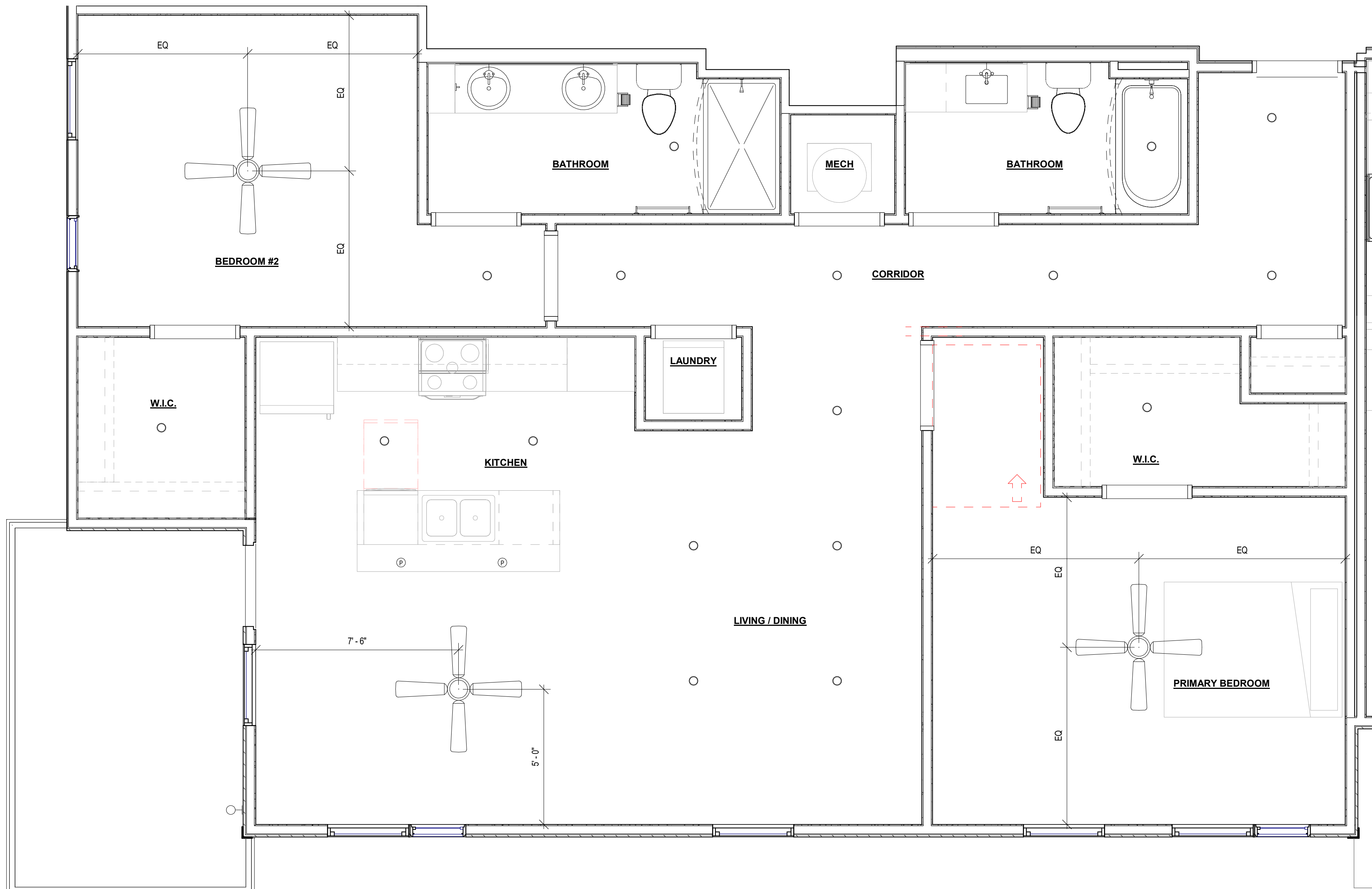
F7 UNIT C2 - REFLECTED CEILING PLAN 3/8" = 1'-0"
