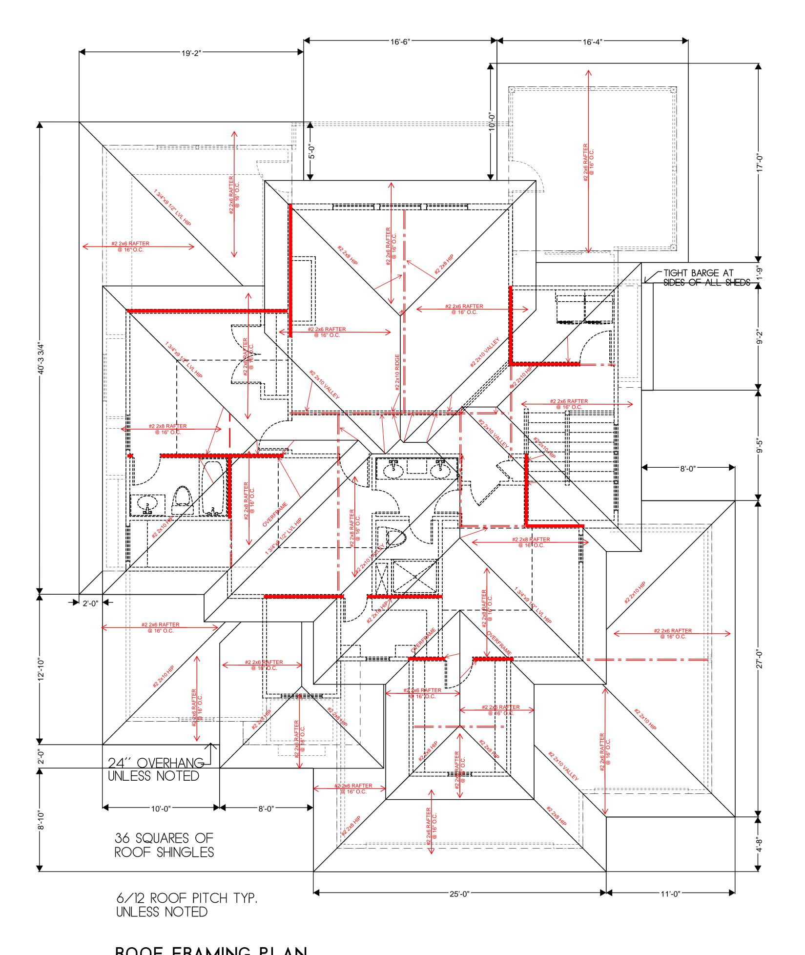
ROOF DESIGNED FOR LIGHT ROOF COVERING 30PSF
