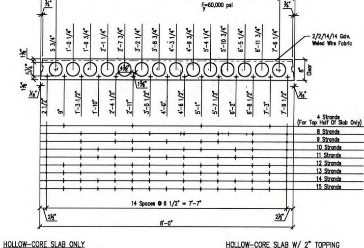
$A = 470 \text{ in}^2$ Wt. = 61.2 psf  $1 = 3525 \text{ in}^4$ b = 27.75 in  $Y_{x} = 4.04$  in  $Y_{b} = 3.96$  in  $Z_{z} = 873$  in  $Y_{z} = 890$  in  $Y_$
