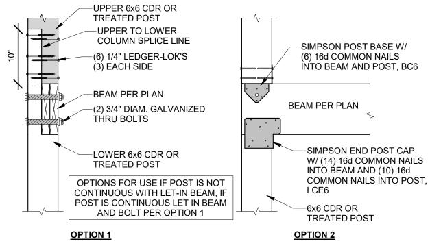
DECK LEVEL EXTERIOR BEAM TO COLUMN
