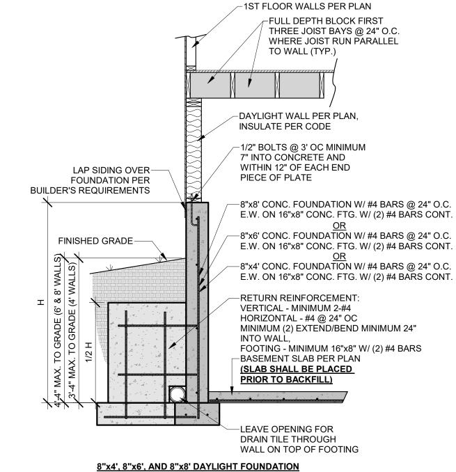
IF SLAB IS NOT PLACED PRIOR TO BACKFILL CONTRACTOR IS RESPONSIBLE FOR BRACING THE FOUNDATION AS REQUIRED
