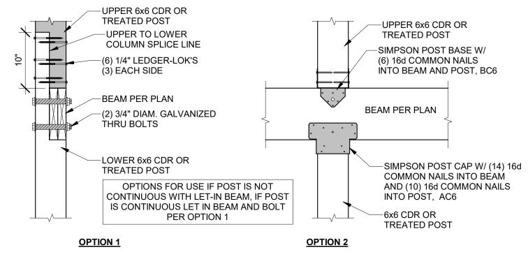
DECK LEVEL INTERIOR BEAM TO COLUMN
