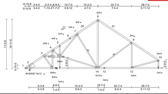
Plate Offsets (X, Y): [3:0-2-6,0-3-0], [10:Edge,0-0-12], [11:Edge,0-2-8], [12:0-2-8,0-1-8], [14:0-4-8,0-2-0], [16:0-3-8,Edge], [17:0-3-0,Edge], [19:0-2-11,0-4-0]
