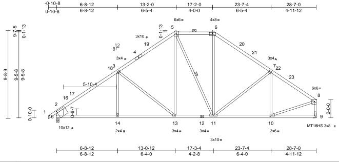
Plate Offsets (X, Y): [5:0-3-5,Edge], [6:0-4-0,0-1-9], [8:0-2-8,Edge], [9:0-3-8,Edge], [10:0-2-8,0-1-8], [15:0-2-11,0-4-0]
