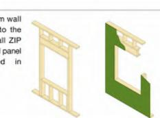
4. Cut two pieces of ZIP System tape or another adhesive-backed flashing tape (must meet ICC-ES Acceptance Criteria for Flashing Materials (AC148)) and apply to each of the window jamb flanges, ensuring the jamb flashings overlap the sill flashing
