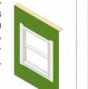
2. If recommended by the window manufacturer, cut a strip of wood to function as a back dam at the sill. The wood strip should have a length equal to the width of the rough opening and a height and width of at least 1/2". Position the block at the inside edge of the window frame.
