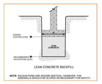
The footings could also bear on properly compacted backfill extending down to suitable soils as shown in the following figure. Overexcavation for compacted engineered fill placement below footings should extend laterally beyond all edges of the footings at least 8 inches per foot of overexcavation depth below footing elevation. The overexcavation should then be backfilled up
