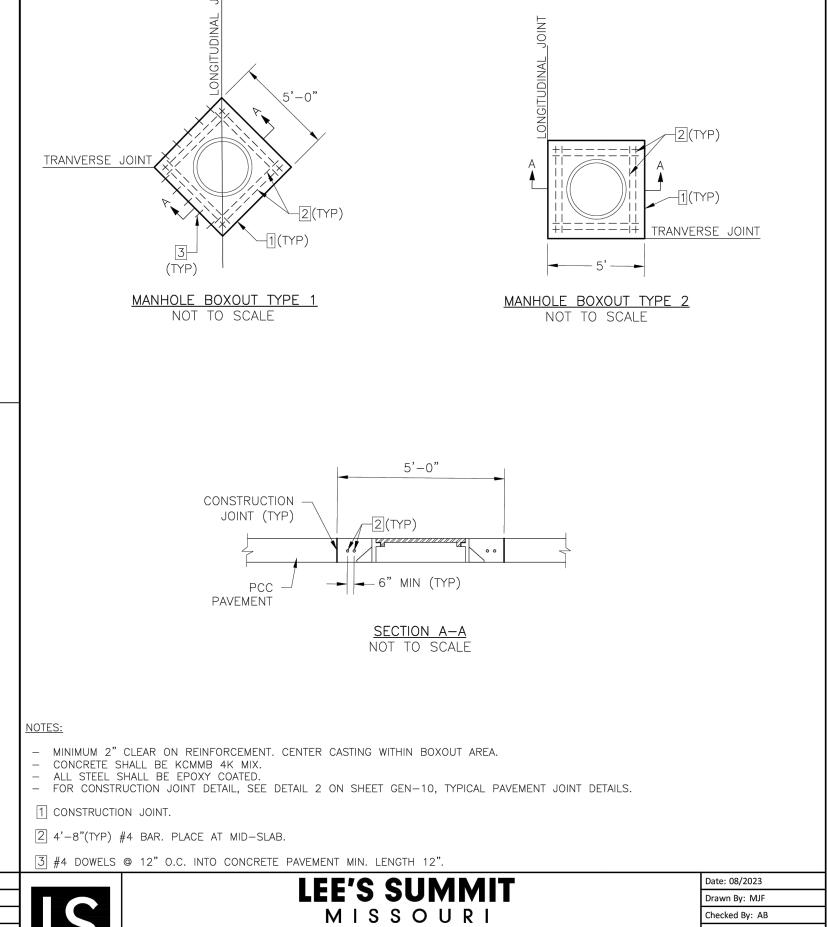
MANHOLE BOXOUT IN PAVEMENT DETAIL
