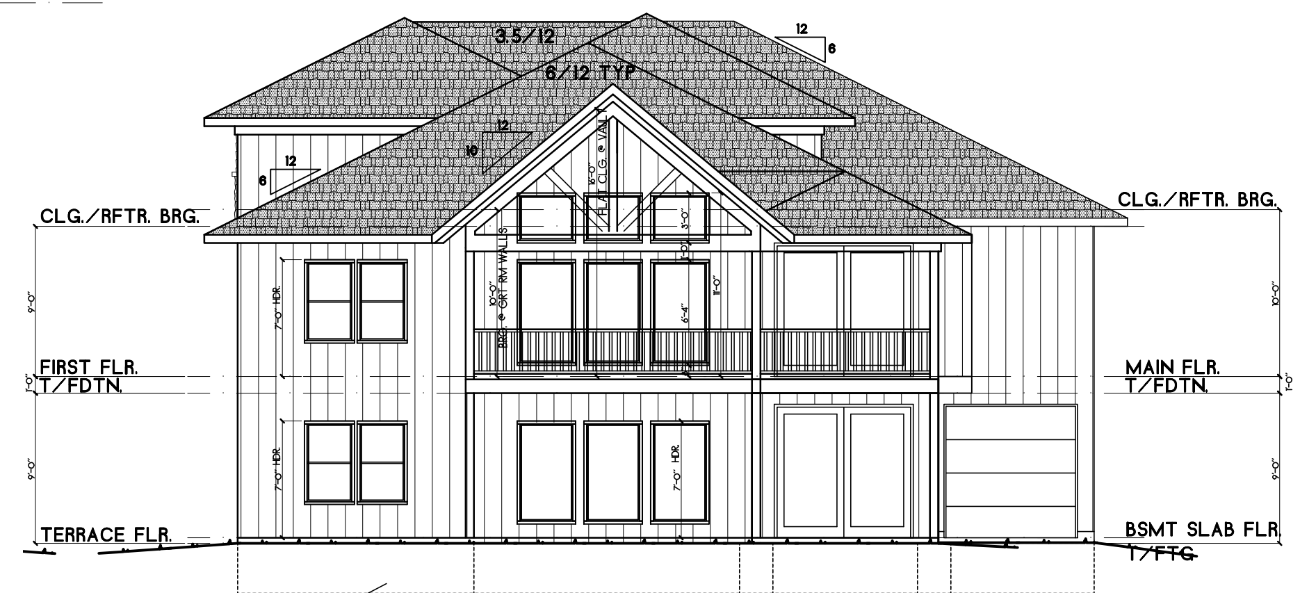
REAR ELEVATION SCALE 1/4"=1'-0"
