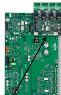
Model PAD-5-CDC Mounted to a PAD-5-MB Main Board
