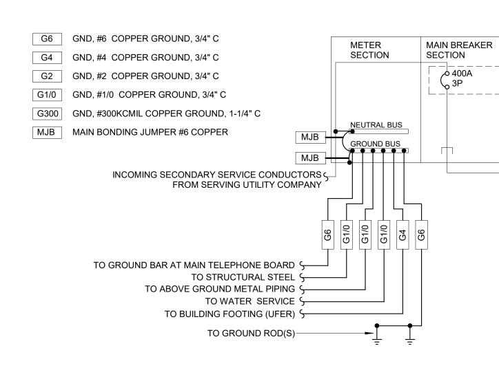
4 GROUNDING ELECTRODE SYSTEM DETAIL
