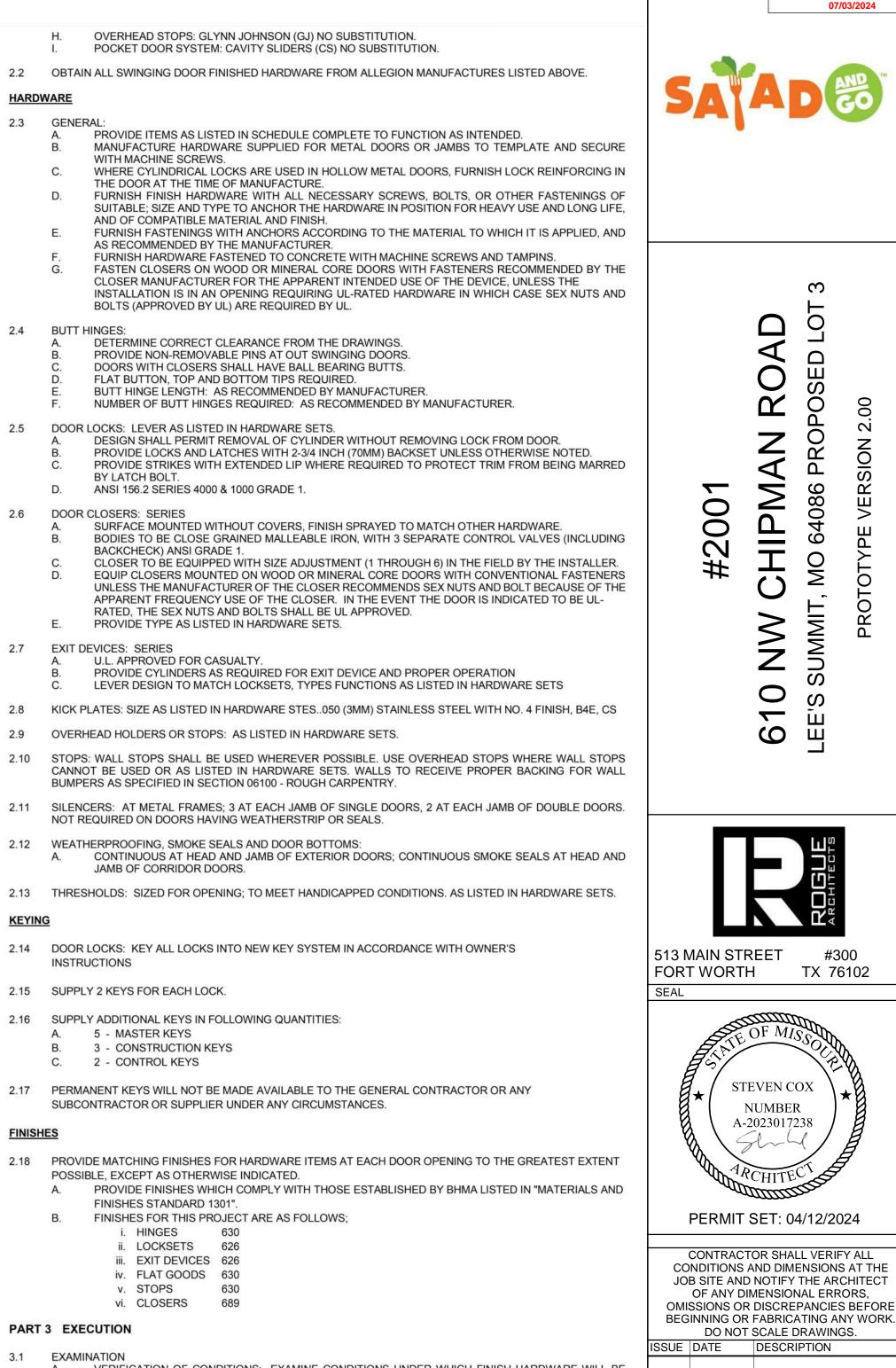
VERIFICATION OF CONDITIONS: EXAMINE CONDITIONS UNDER WHICH FINISH HARDWARE WILL BE INSTALLED. REPORT DEFICIENCIES TO THE ARCHITECT.
