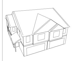
TRUSS QUANTITY 89 **GABLE AREA** 785 HIP LINES 0 115 HORIZONTAL OVERHANG LINES 207 RAKED OVERHANG LINES RIDGE LINES 79 **ROOF AREA** 3,105 VALLEY LINES 53
