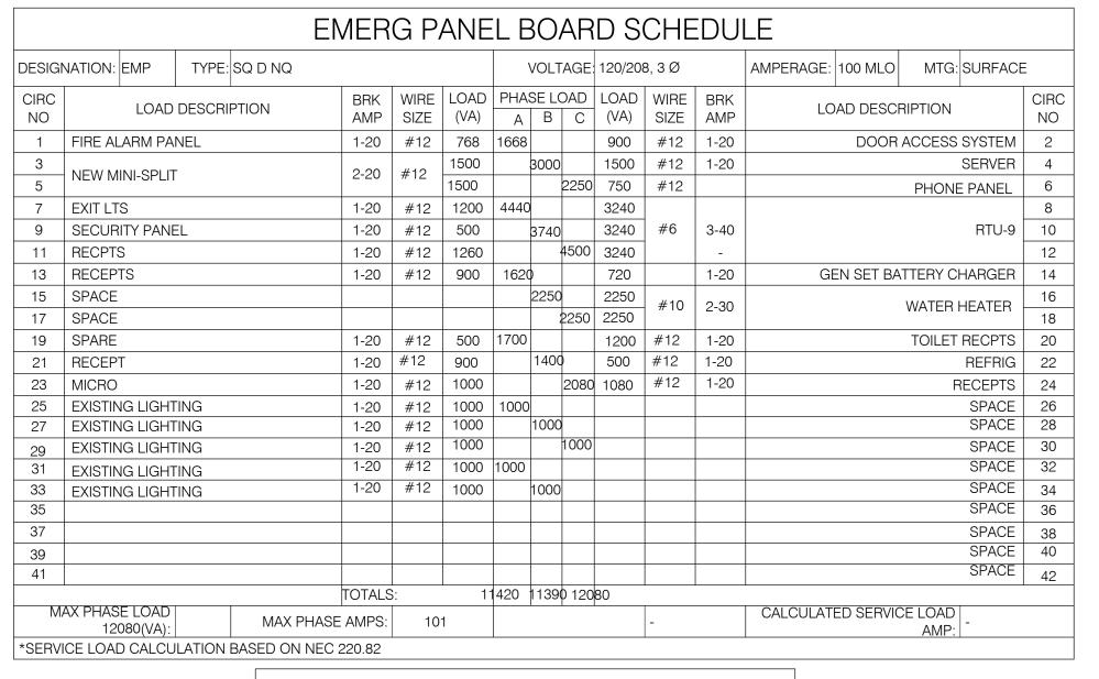
RELOCATE EXISTING LIGHTING CIRCS FROM EXISTING PANEL B TO EMERG PANEL. COMBINE CIRCUITS ONTO BRKRS (EMERG-25-33), EQUALIZE WATTAGE AS CLOSE AS POSSIBLE, TOTAL WATTAGE SHOULD BE APPROX. 4500W.
