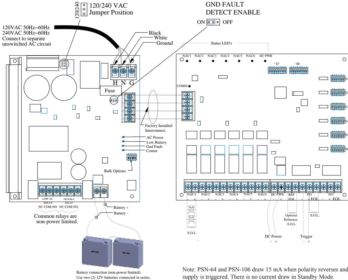
Note: PSN-64 and PSN-106 draw 15 mA when polarity reverses and the power supply is triggered. There is no current draw in Standby Mode.
