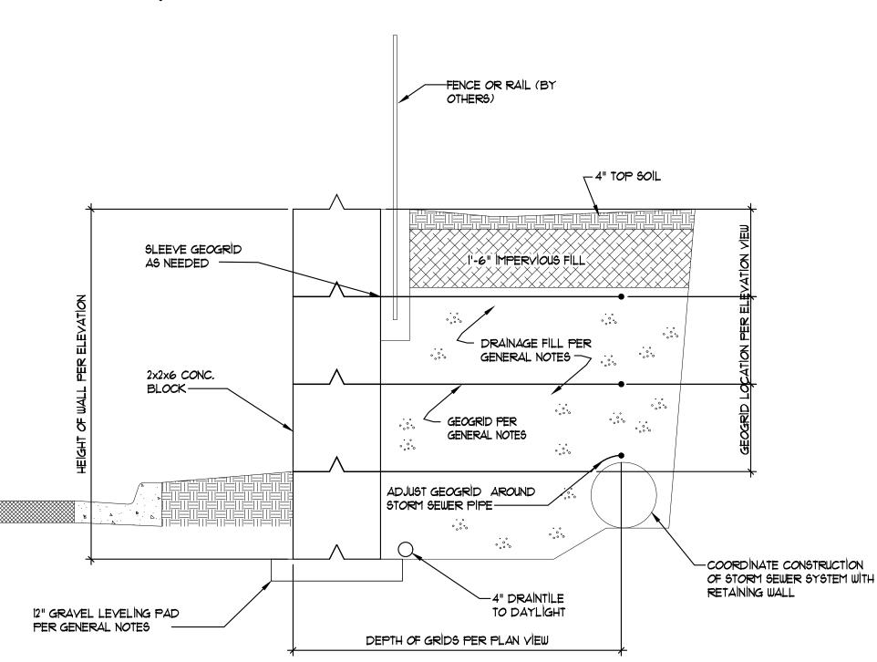
REINFORCED SOIL RETAINING WALL SECTION SCALE: 1/2" = 1'-0"
