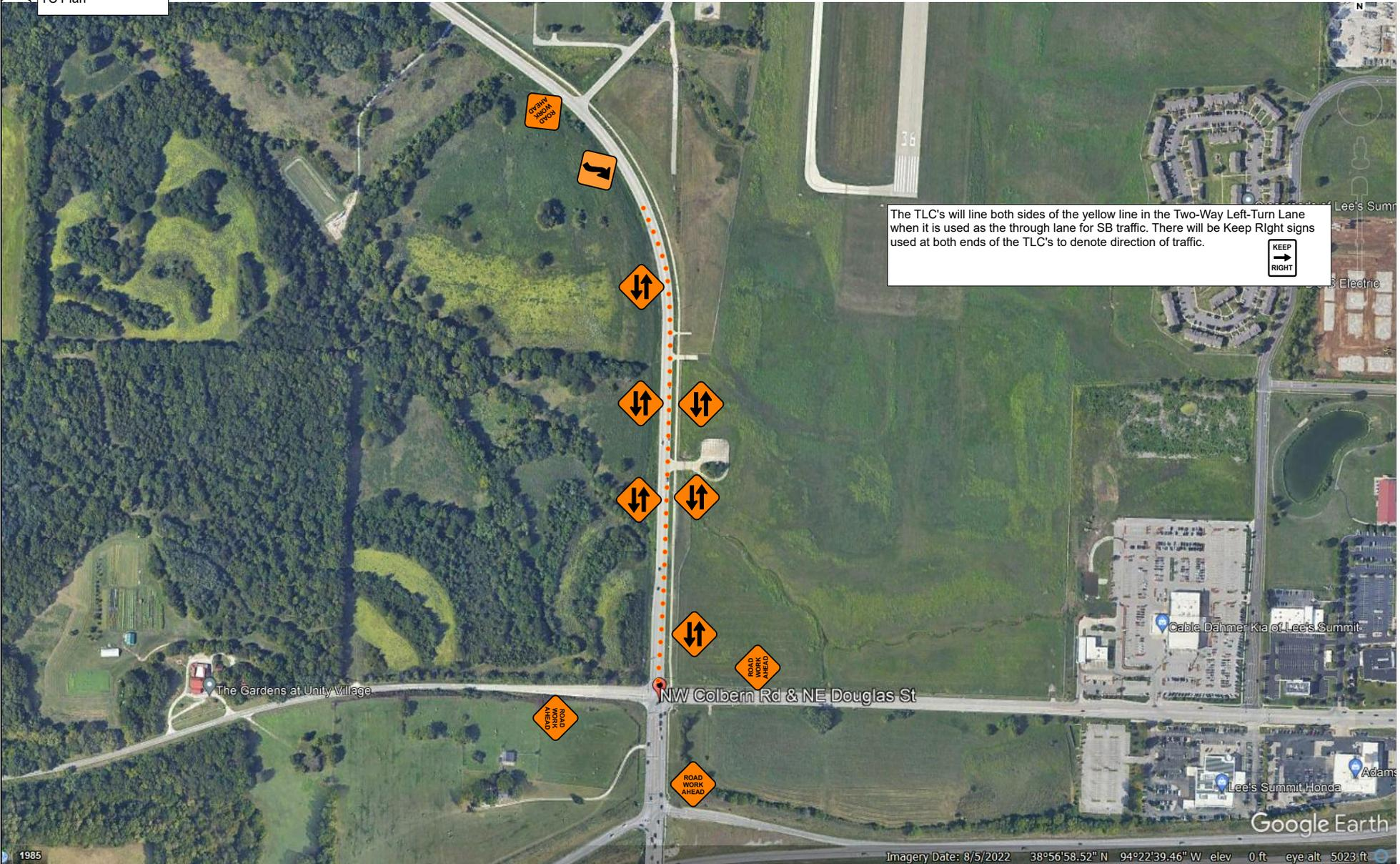
The TLC's will line both sides of the yellow line in the Two-Way Left-Turn Lane when it is used as the through lane for SB traffic. There will be Keep Right signs used at both ends of the TLC's to denote direction of traffic.
