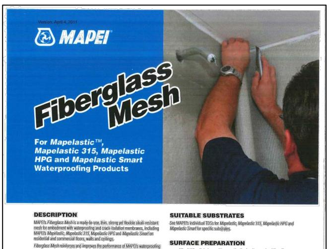
SURFACE PREPARATION All suitable substrates must be smooth, structurally sound and free of any membranes when applied over cracks, coves and corners and around drains on residential and commercial applications. Fiberglass Mesh can be cut to size with substance that could prevent adhesion. scissors or a razor knife, and has excellent compatibility with all MAPEI cement- or
