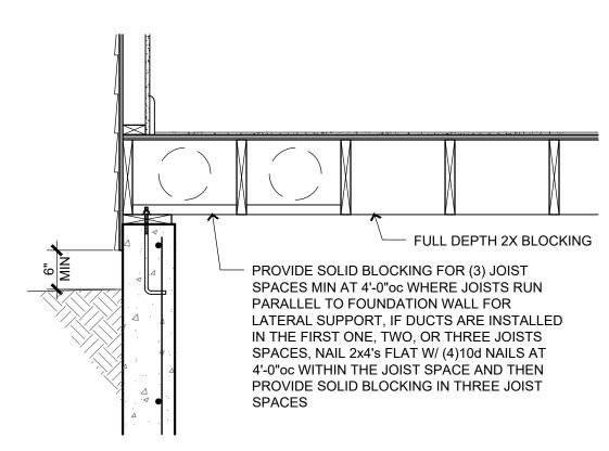
JOISTS PARALLEL TO WALL SCALE: 3/4" = 1'-0"
