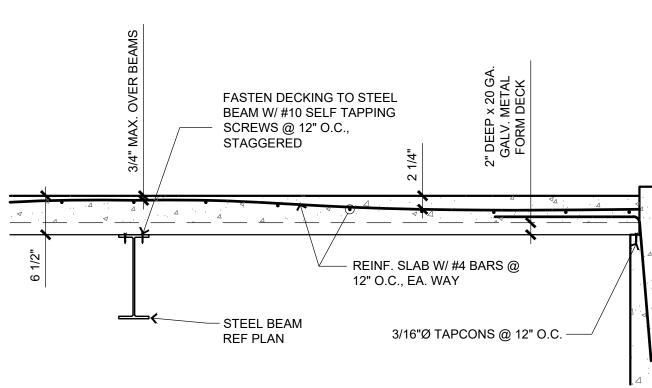
**SLAB OVER BEAM** SCALE: 3/4" = 1'-0"
