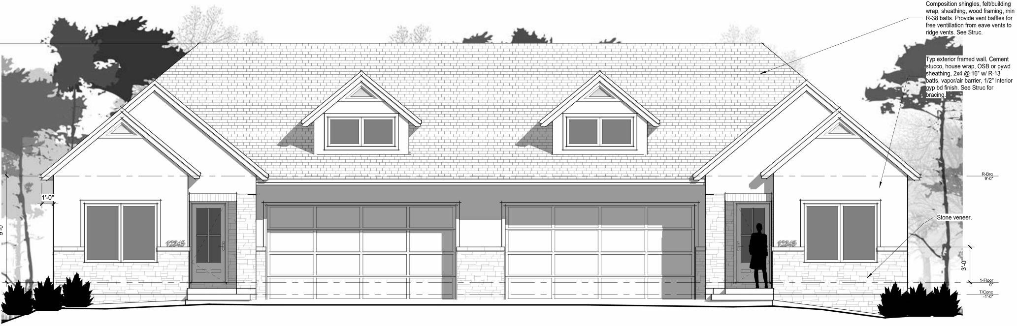
Composition shingles, felt/building wrap, sheathing, wood framing, min
