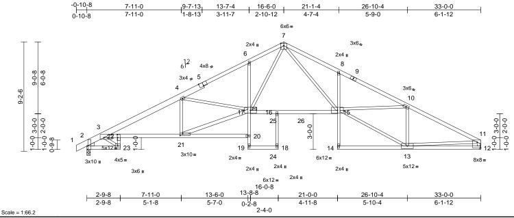
Plate Offsets (X, Y): [2:0-3-8,Edge], [3:0-8-0,0-3-2], [5:0-4-0,Edge], [12:Edge,0-5-13], [21:0-2-8,0-1-8], [22:0-3-0,0-0-8]
