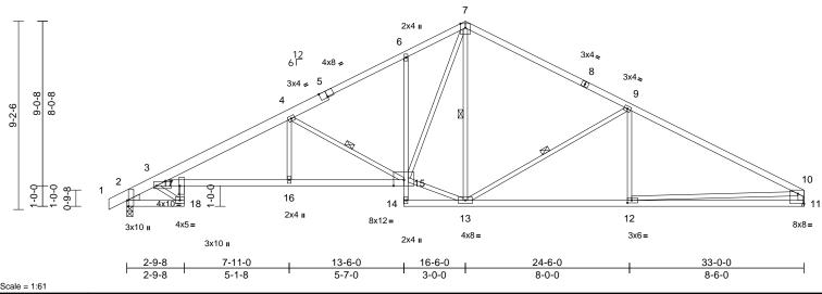
Plate Offsets (X, Y): [2:0-3-8,Edge], [3:0-8-8,0-2-6], [5:0-4-0,Edge], [11:Edge,0-5-13], [12:0-2-8,0-1-8], [17:0-5-0,0-0-8]
