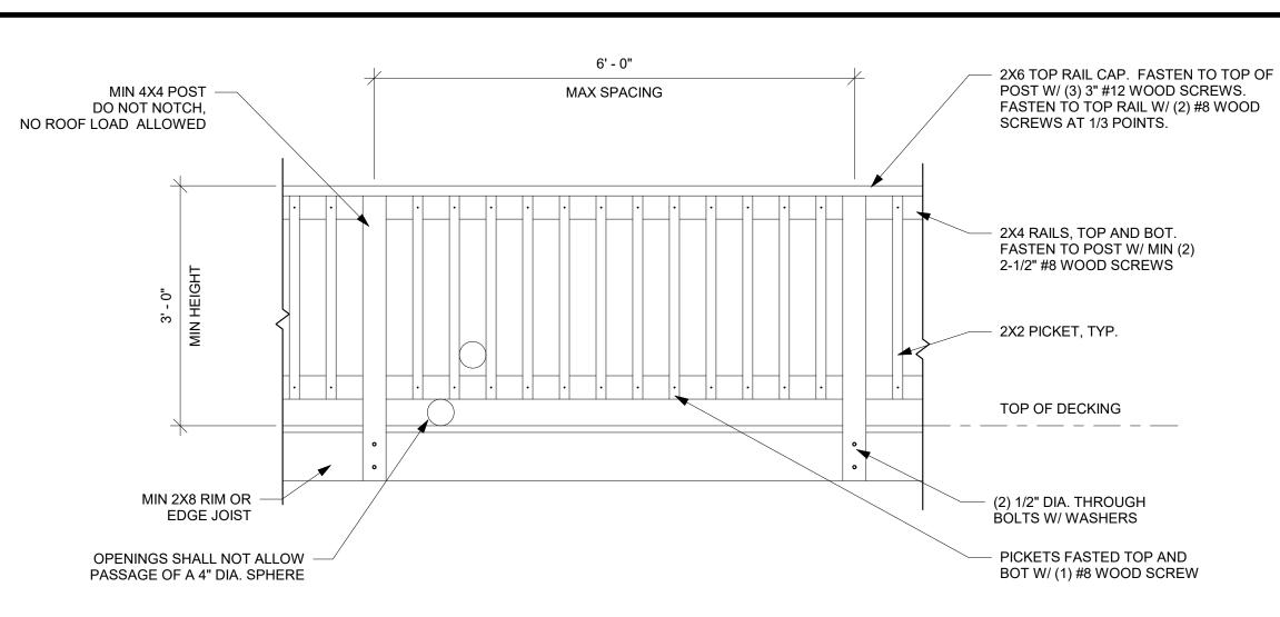
DECK RAILING DETAIL DRAWN TO MEET THE INTENT OF R312 OF THE 2018 IRC AND A CONCENTRATED LOAD OF 200 LBS PER 1607.8.1 OF THE 2018 IBC.
