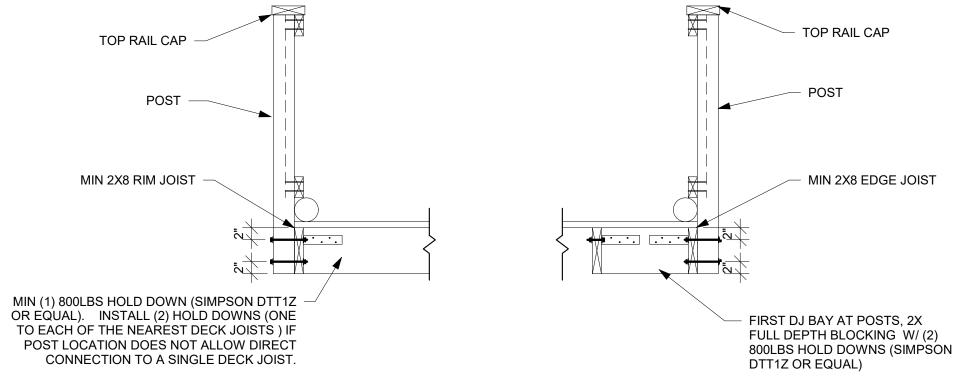
**RAILING ATTACHED TO RIM JOIST**
