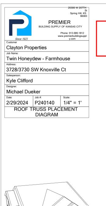
TRUSS QUANTITY 89 **GABLE AREA** 785 HIP LINES 0 115 HORIZONTAL OVERHANG LINES 207 RAKED OVERHANG LINES RIDGE LINES 79 **ROOF AREA** 3,105 VALLEY LINES 53
