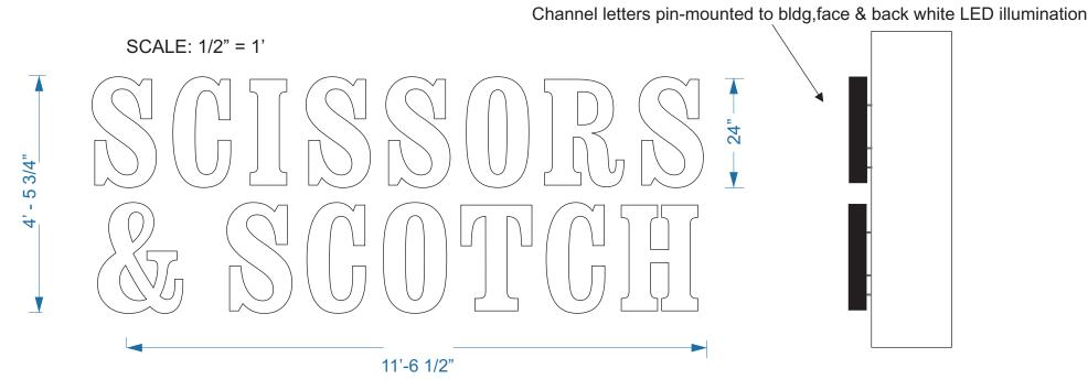
**Channel Letter & Wall Cross Section** Flush Mounted, Backer, Interior Power Supplies Letters Front and Rear Iluminated Clear Acrylic Primary Electrical Trimcap Service Switch 2"x4" LED's Electrical Вох Power Supply, mounted to .080" backer – Face Mounting, Wall appropriate for wall type. Return Backer Panel
