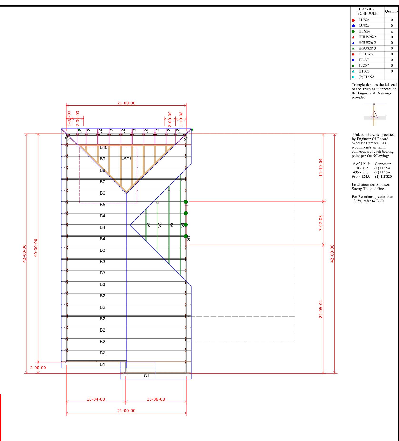
Roof Truss Layout Scale: 1/4" = 1'
