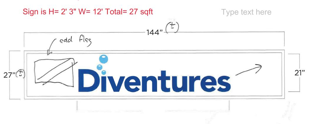
NEW WHITE POLYCARBONATE FACE 3M 3630-167 BLUE 'DIVENTURES' LETTERING 3M 3630-57 PROCESS BLUE 'BUBBLES' SIGN FACE TO INSTALL IN EXISTING CABINET NO ELECTRICAL REQUESTED
