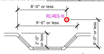
If additional floor area is created. Cannot exceed 18 ft<sup>2</sup>, be more than 2'-0" deep, more than 9'-0" wide and be with in the coverage area of the sprinkler. No Additional Sprinkler is Required.
