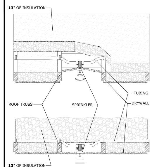
From the <u>Uponor AquaSAFE Attic Insulation Guidelines</u> we use the following formula for the recommended minimum amount of insulation required on top of our pipe for figure 2 alternative installation.
