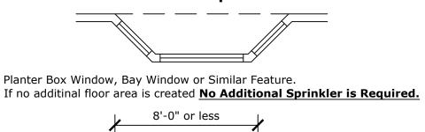
If no additinal floor area is created No Additional Sprinkler is Required.
