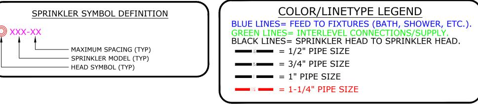
SENJU Model RC-RESLF37 LowFlow K3.7 Residential Concealed Pendent SS8261 K=3.7, 162F°, 7/16" Orifice, Maximum Spacing 16'x16' Sprinkler head demand: 14 gpm @ 14.3
