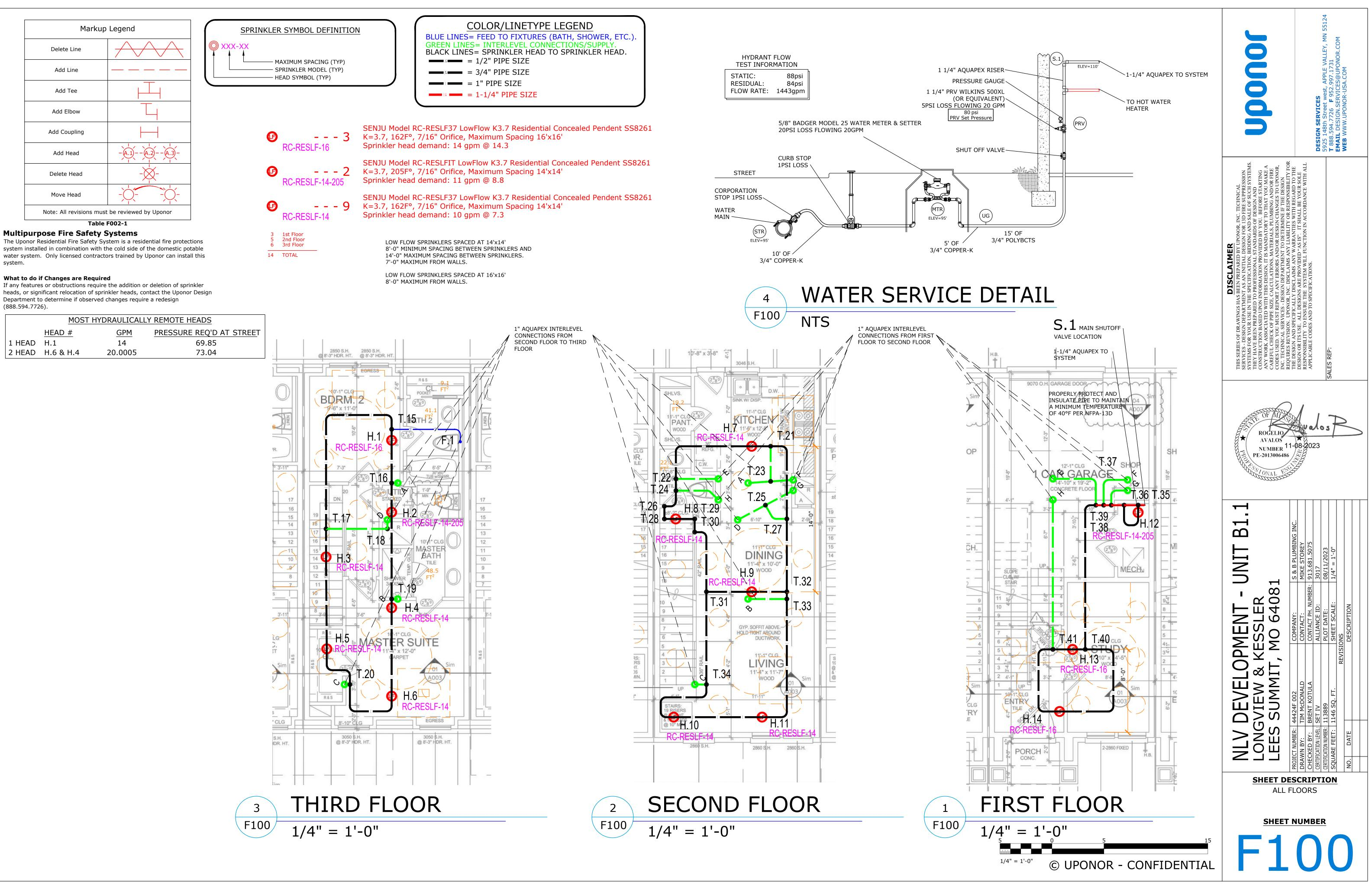
The Uponor Residential Fire Safety System is a residential fire protections system installed in combination with the cold side of the domestic potable water system. Only licensed contractors trained by Uponor can install this system.
