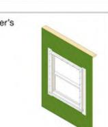
7. Cut a piece of rigid head flashing so that when installed, it is flush with the edges of the exterior moulding of the window. Apply a bead of sealant to the back and bottom surface of the rigid head flashing. Use sealant recommended by the flashing manufacturer.
