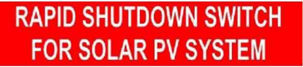
LABEL 12 A RAPID SHUTDOWN SWITCH SHALL HAVE A LABEL LOCATED ON OR NO MORE THAN 1M (3FT) FROM THE SWITCH THAT INCLUDES THE FOLLOWING WORDING "RAPID SHUTDOWN SWITCH FOR SOLAR PV SYSTEM" THE LABEL SHALL BE REFLECTIVE WITH ALL LETTERS CAPITALIZED AND HAVING A MINIMUM HEIGHT OF 9.5MM (3/8 IN.), IN WHITE ON RED BACKGROUND)
