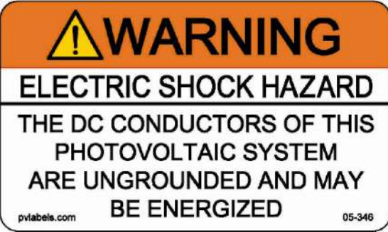
LABEL 1 AT EACH JUNCTION BOX, COMBINER BOX, DISCONNECT, AND DEVICE WHERE ENERGIZED UNGROUNDED CONDUCTORS MAY BE EXPOSED DURING SERVICE. NEC. 690.35(F)
