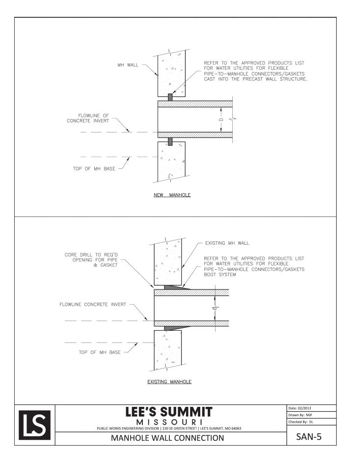
6 MANHOLE WALL CONNECTION (C501) N.T.S.
