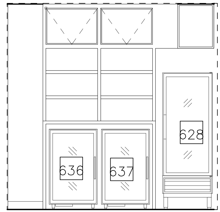
IN A PINCH EQUIPMENT ELEVATION WITH BEER AND WINE SERVICE 1/2" = 1'-0"
