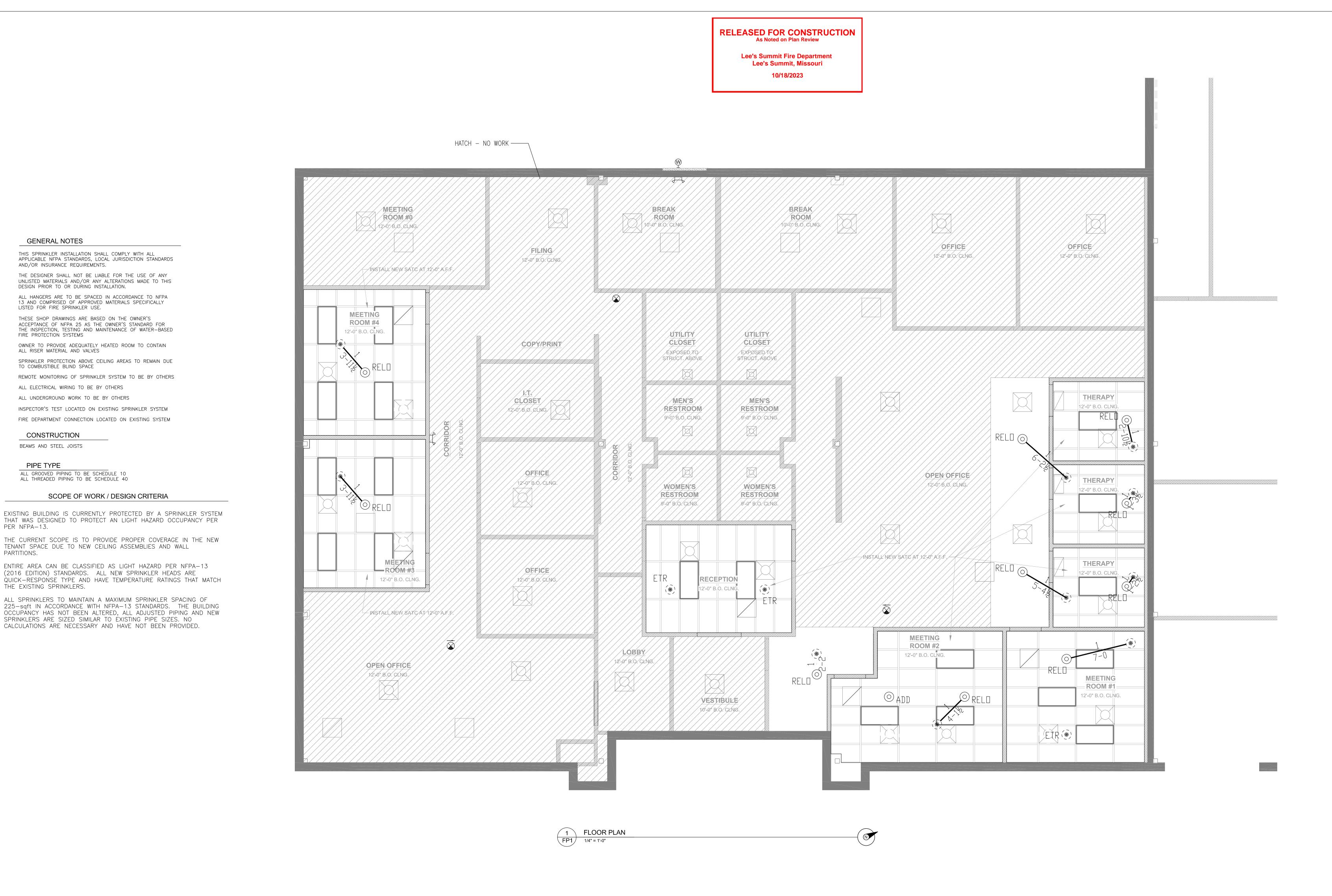
ALL HANGERS ARE TO BE SPACED IN ACCORDANCE TO NFPA 13 AND COMPRISED OF APPROVED MATERIALS SPECIFICALLY LISTED FOR FIRE PROTECTION USE. ALL PENDENT SPRINKLER ARMOVERS GREATER THAN 12" SHALL BE SUPPORTED BY AN NFPA
