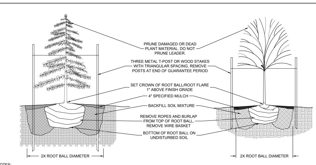
1. IN TURF AREA, PROVIDE 6' DIAMETER OF MULCH
