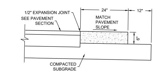
1. 3/4" ISOLATION JOINTS WITH 5/8" DIA. X 2' SMOOTH DOWELS SHALL BE PLACED AT RADIUS POINTS AND AT 150' INTERVALS. THESE DOWEL BARS SHALL BE GREASED AND WRAPPED ON ONE END WITH EXPANSION TUBES. 2. 1" DEEP CONTRACTION JOINTS SHALL BE INSTALLED AT APPROXIMATELY 10' INTERVALS. THESE JOINTS SHALL PASS ACROSS THE ENTIRE CURB SECTION.
