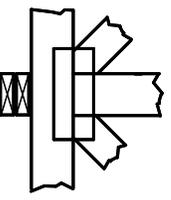
Indicates location where bearings (supports) occur. Icons vary but reaction section indicates joint number/letter where bearings occur. Min size shown is for crushing only.
