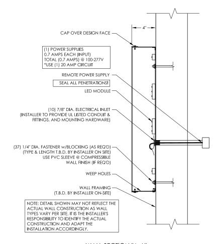
WALL SECTION "A-A" SCALE 1:8
