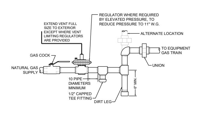
**GAS EQUIPMENT CONNECTION DETAIL** NO SCALE
