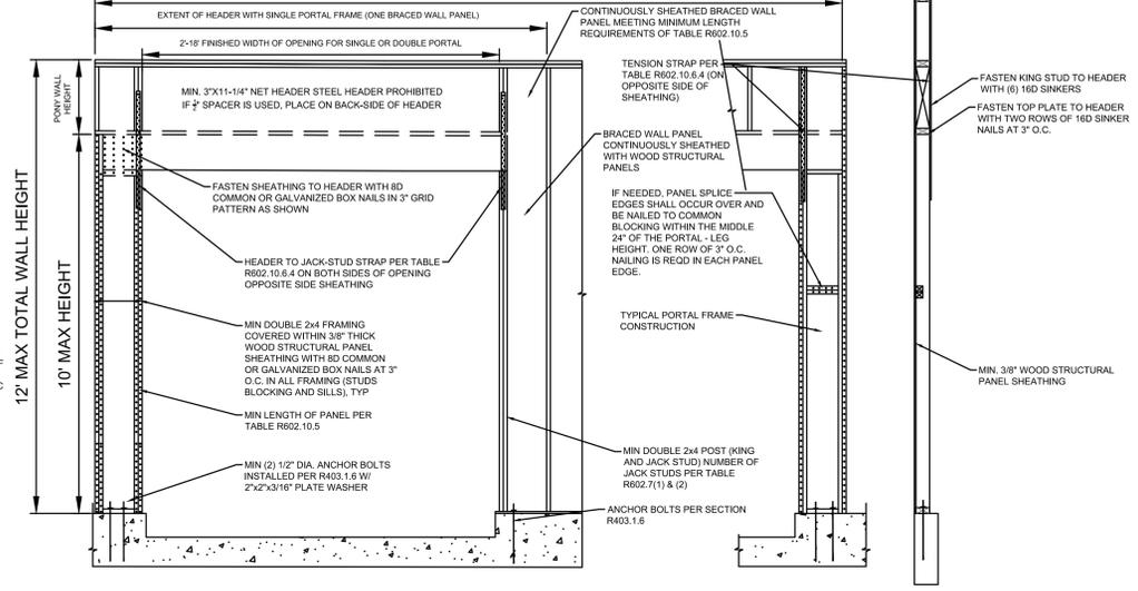
13 METHOD CS-PF - CONTINUOUSLY SHEATHED PORTAL FRAME PANEL CONSTRUCTION (IRC FIGURE R602.10.6.4) N.T.S.
