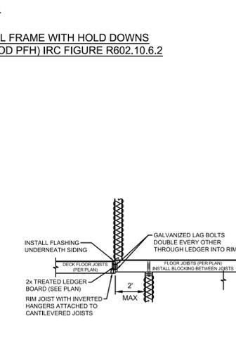
10 TYPICAL CANTILEVER FRAMING WITH DECK ATTACHMENT N.T.S.
