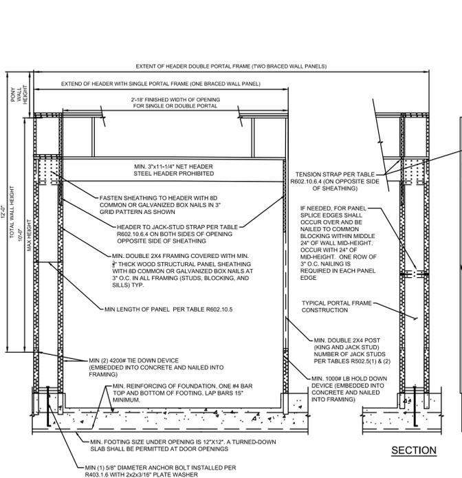
14 PORTAL FRAME WITH HOLD DOWNS (METHOD PFH) IRC FIGURE R602.10.6.2 N.T.S.
