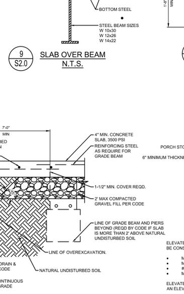
3 TYPICAL FOOTING/FOUNDATION WALL STANDARD SLAB AT MAX 4" OVERDIG N.T.S.
