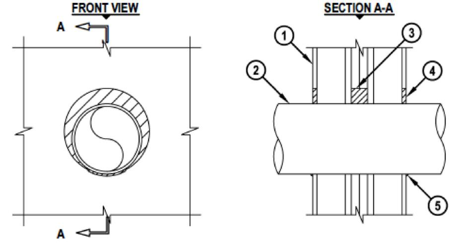
1. GYPSUM WALL ASSEMBLY (UL/cUL CLASSIFIED U300 SERIES) (2-HR. FIRE-RATING) CONSISTING OF THE FOLLOWING :
