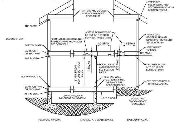
15 TYPICAL WALL, FLOOR AND ROOF FRAMING (IRC FIGURE R602.3(1)) N.T.S.
