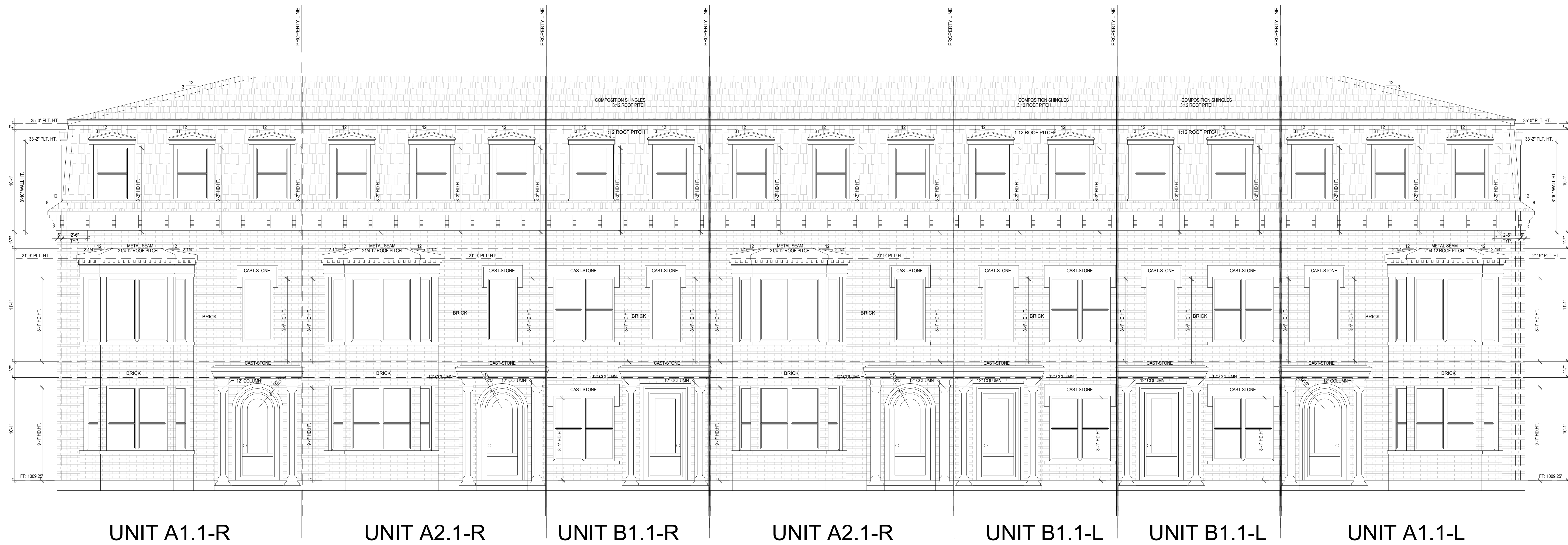
02 | BUILDING 2 - FRONT ELEVATION 1/4" = 1'-0"
