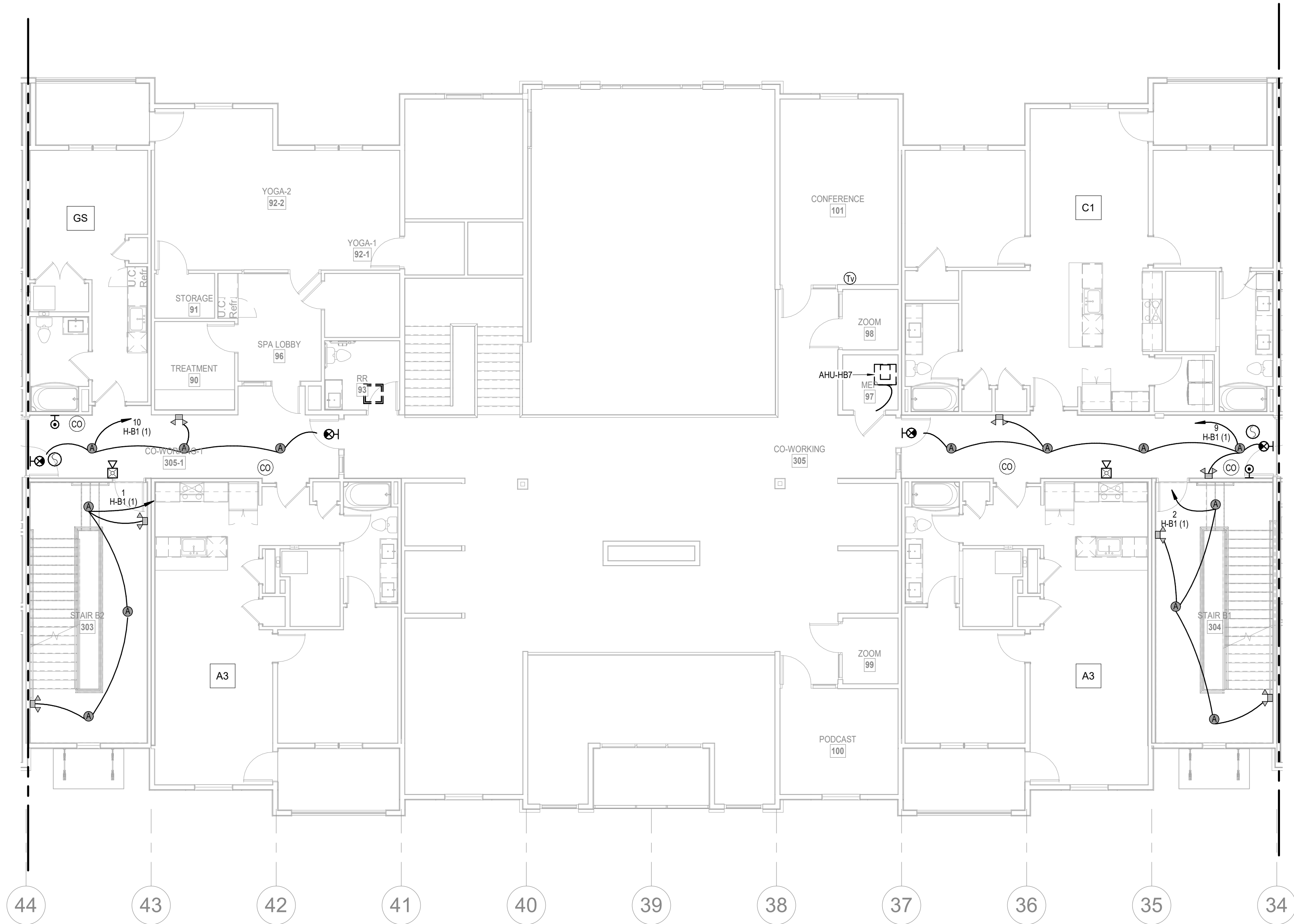
2 2ND FLOOR - SEGMENT B ELECTRICAL 1/8" = 1'-0"
