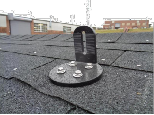
Photo No. 2 Nano Deck Mounted Test Specimen
