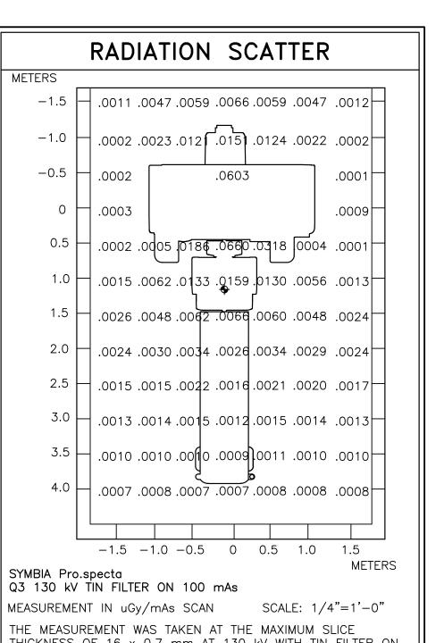
THICKNESS OF 16 x 0.7 mm AT 130 kV WITH TIN FILTER ON AND 100 mAs/scan IN THE HORIZONTAL PLANE THROUGH THE SYSTEM AXIS. THE PHANTOM USED WAS A CYLINDRICAL PMMA PHANTOM WITH A DIAMETER OF 32 CM AND A LENGTH OF 16 CM. THE PHANTOM WAS CENTERED IN THE TOMOGRAPHIC - INDICATES SPECT ORIENTATION POINT
