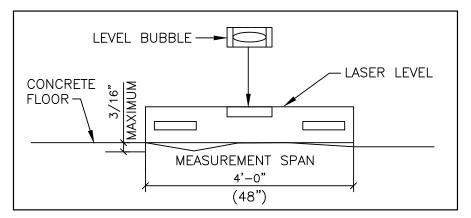
IT IS THE CUSTOMER/CONTRACTOR'S RESPONSIBILITY THAT ANY MEASUREMENT OUT OF ACCEPTABLE LIMITS ARE AN INDICATION THAT THE FLOOR NEEDS TO BE RELEVELED.
