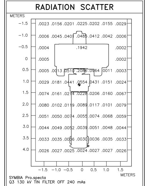
MEASUREMENT IN uGy/mAs SCAN SCALE: 1/4"=1'-0"THE MEASUREMENT WAS TAKEN AT THE MAXIMUM SLICE THICKNESS OF 16 x 0.7 mm AT 130 kV WITH TIN FILTER ON AND 240 mAs/scan IN THE HORIZONTAL PLANE THROUGH THE SYSTEM AXIS. THE PHANTOM USED WAS A CYLINDRICAL PMMA PHANTOM WITH A DIAMETER OF 32 CM AND A LENGTH OF 16 CM. THE PHANTOM WAS CENTERED IN THE TOMOGRAPHIC PLANE. INDICATES SPECT ORIENTATION POINT
