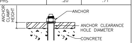
ANCHOR CLAMP HEIGHT IS THE DISTANCE FROM THE FINISHED FLOOR TO THE TOP OF THE FIXTURE BEING CLAMPED.
