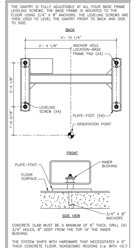
SDS VALUES) MAY HAVE FLOORS THAT ARE LESS THAN 6" THICK. CUSTOMER'S IS RESPONSIBLE TO CONSULT THE ENGINEER OF RECORD FOR THE BUILDING FOR SPECIFIC
