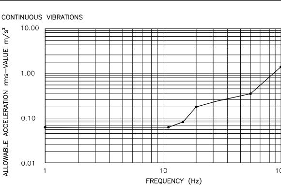
EXTERNAL VIBRATIONS OR SHOCK TRANSMITTED BY THE WALLS OR FLOOR OF THE BUILDING MAY AFFECT THE GANTRY AND DEGRADE IMAGE QUALITY OF THE SYMIBA SYSTEM. THEREFORE THE GANTRY AND THE PATIENT HANDLING TABLE MUST BE INSTALLED IN AN ENVIRONMENT FREE OF VIBRATIONS. SOURCES THAT PRODUCE VIBRATIONS ARE RAILROADS, SUBWAYS, ROADS, CONSTRUCTION, POWER PLANTS, MINES, FERRY MOORINGS, AND ANY OTHER SOURCE STRIKING VIBRATIONS.
