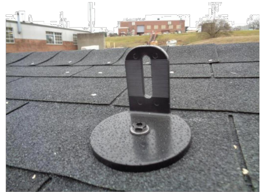
Photo No. 3 Nano Rafter Mounted Test Specimen
