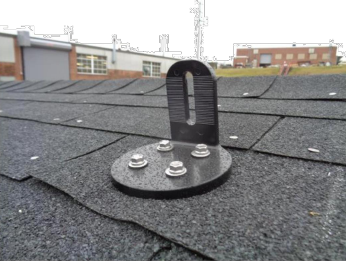
Photo No. 2 Nano Deck Mounted Test Specimen
