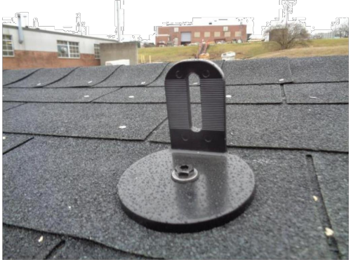
Photo No. 3 Nano Rafter Mounted Test Specimen
