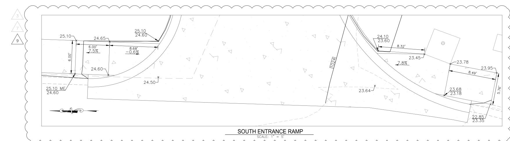
NOTE: INSTALL FORM BOARD AT STRUCTURE OPENING AND POUR SIDEWALK AGAINST IT. 5' MINIMUM
