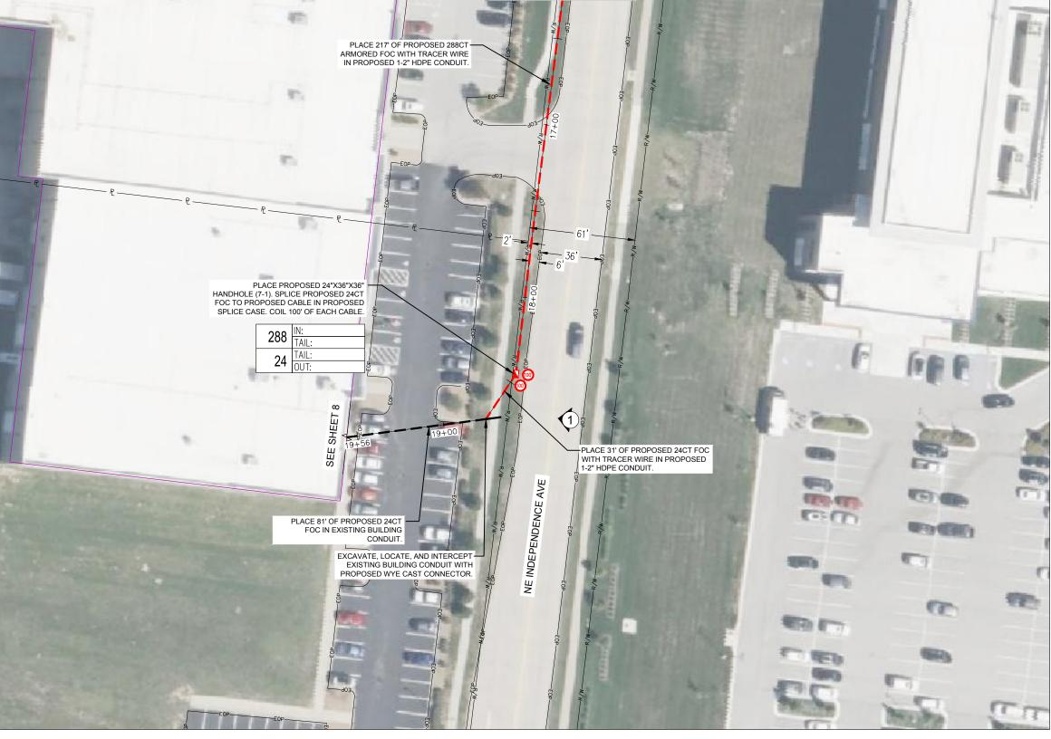
LOCATE EXISTING BUILDING CONDUIT BEFORE BEGINNING CONSTRUCTION.
