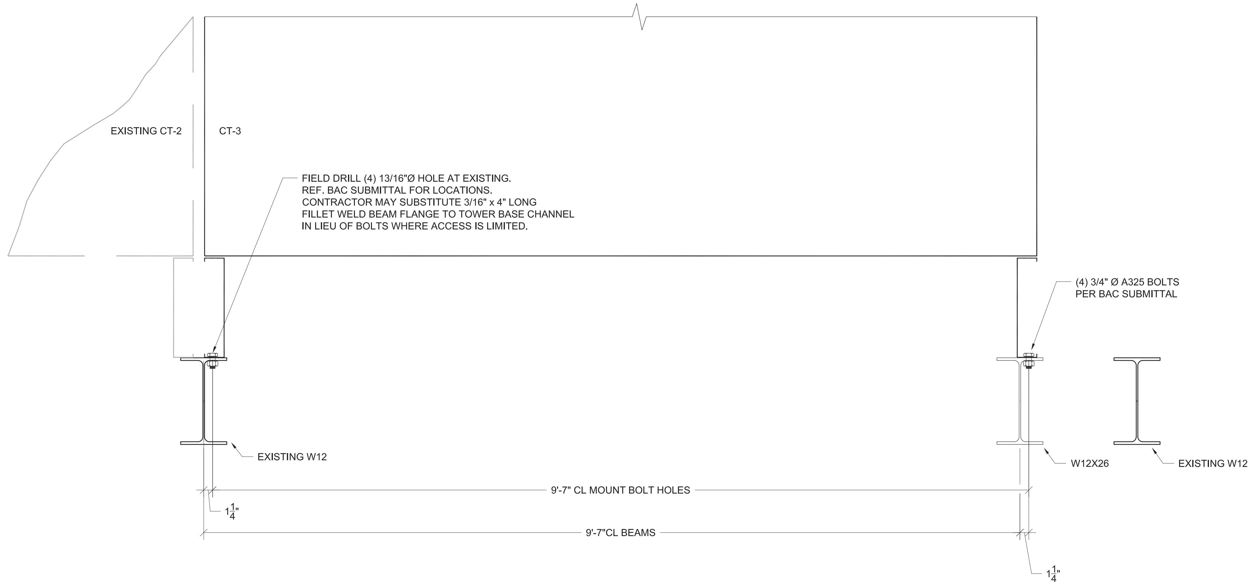
7 SECTION AT TOWER MOUNTS SCALE: 1 1/2"=1'-0"
