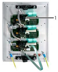
Figure 19. SK enclosure integrated wall control unit with keypad, interior
