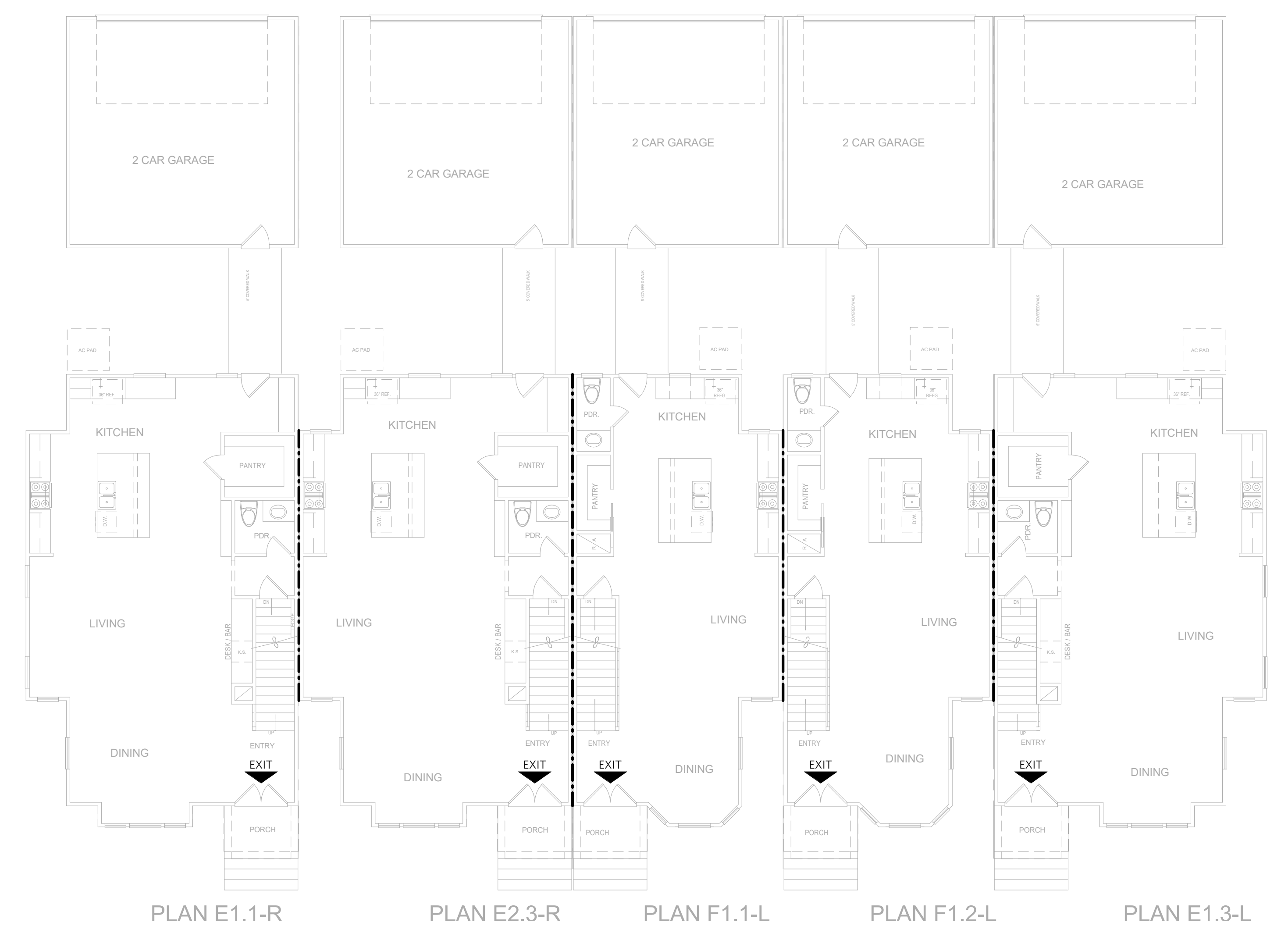
05 | BUILDING 4 - FIRST FLOOR CODE PLAN 1/8" = 1'-0"
