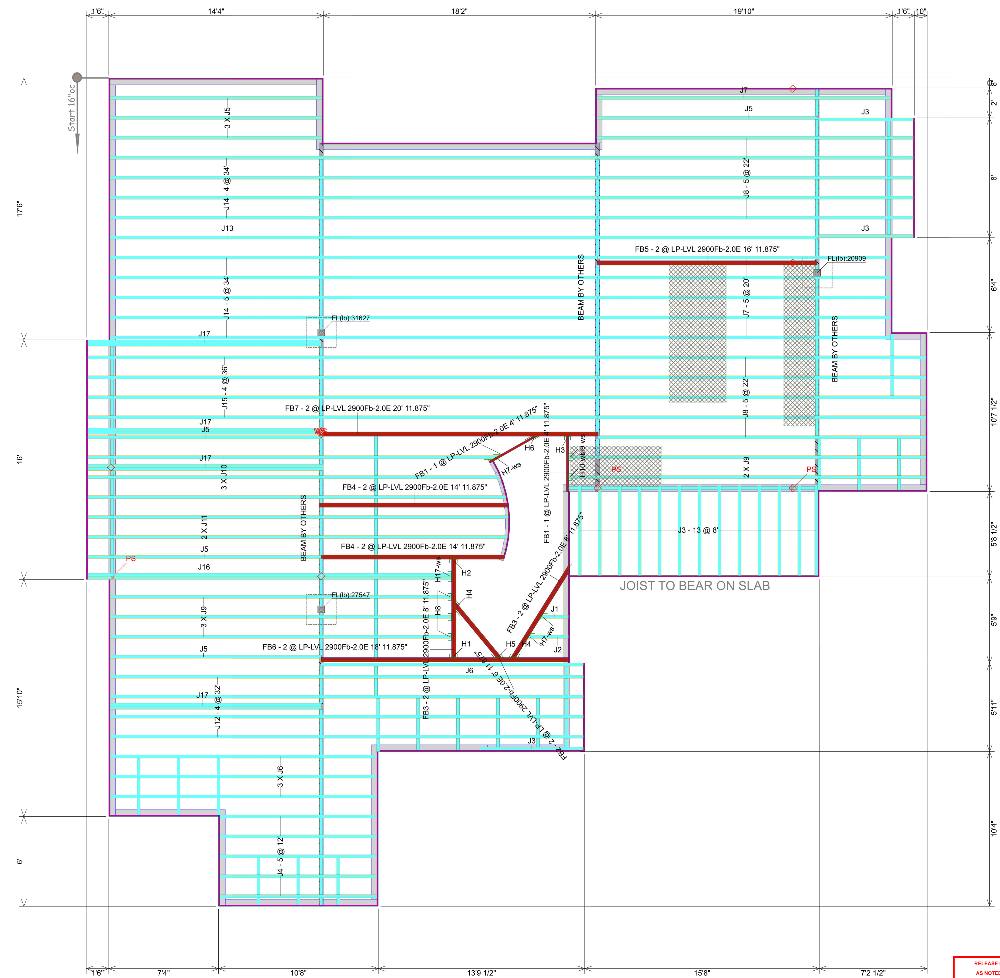
FIRST FLOOR JOIST PLACEMENT PLAN LOT 134 - WOODSIDE RIDGE TL22076ATH
