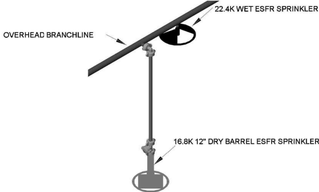
DRY BARREL OVERHEAD CONNECTION N.T.S.
