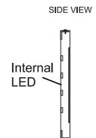
2.0" deep sign cabinet fabricated from aluminum extrusion with black sides, and front. Face will be manufactured from aluminum composite. Attached to the wall of the existing bulkhead with a 3/16" dia. threaded tapcon.
